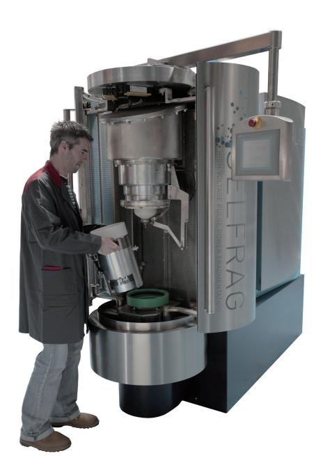
SELFRAG Lab is a laboratory batch equipment. It uses the high voltage pulse power technology of SELFRAG for the selective fragmentation of composite materials, mineralogical, and geological samples in the kilogram range.
